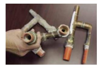
Most recently, Kitec plumbing has become a buzz in the Condominium industry as a result of the North American Class Action Lawsuit regarding the premature failure of the pipes. Although the product was marketed as 'corrosion resistant,' it has been found to fail prematurely due to excessive water pressure or water running at temperatures hotter than the manufacturer's rating of 77C (180F). As a result of these issues the product was recalled in 2005 and is no longer manufactured.
